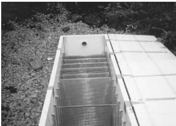
FIGURE 7.11 Filter unit containing filters made of kenaf fiber (USDA).
