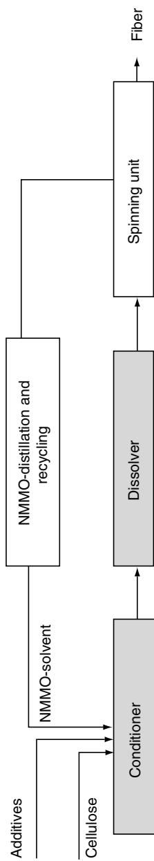
FIGURE 10.17 Block diagram for the continuous dissolution process of cellulose in NMMO. (From Diener, A. and Raouzeos, G., Chem. Fibers Int. , 49(1), 40, 1999. Reprinted with permission of IBP International Business Press.)
