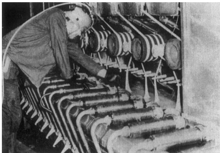
FIGURE 10.71 Viscose rayon spinning machine. (Courtesy of Kemira Oy Sateri, Valkealkoski, Finland.)
