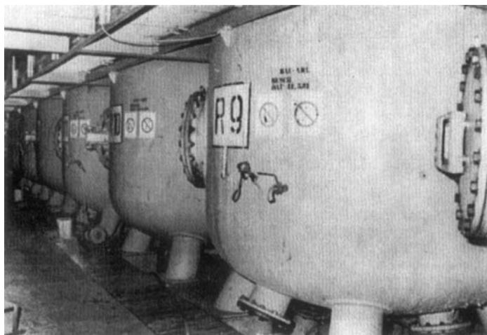
FIGURE 10.70 Viscose ripening tanks. (Courtesy of Chemiefaser Lenzing, A.G. Lenzing, Austria.)
