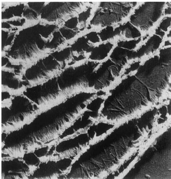
FIGURE 9.49 Portion of thin cross-section showing fibrils in layers of a swelled fiber at higher magnification than Figure 9.48 (TEM).
